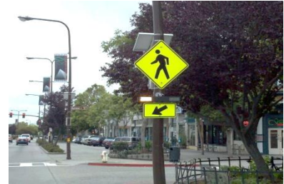
Pedestrian activated lights may be installed on a sign and/or in the pavement.
