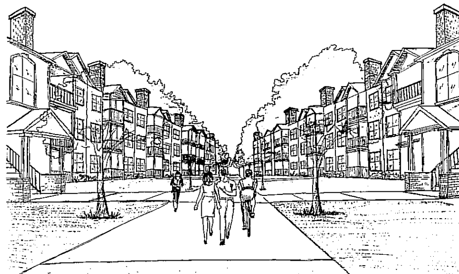
Multi-Family Housing should Emphasize Individual Units to Reduce Mass of the Structure
