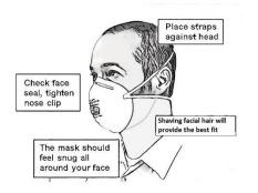
For a respirator that relies on a tight seal to the face, check how well it seals to the face by following the manufacturer's instructions for user seal checks. Adjust the respirator if air leaks between the seal and the face. The more air leaks under the seal, the less protection the user receives.
